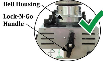
**Step 2:** Lock-N-Go® handles are used for transport. Rotate both handles to a vertical, UNLOCKED, position for use. This allows the bell housing to "float" freely on the springs during operation. **DO NOT operate with handles in the transport position.**
