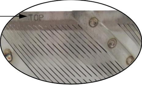
**Element Lead Wire and Retaining Screw**
